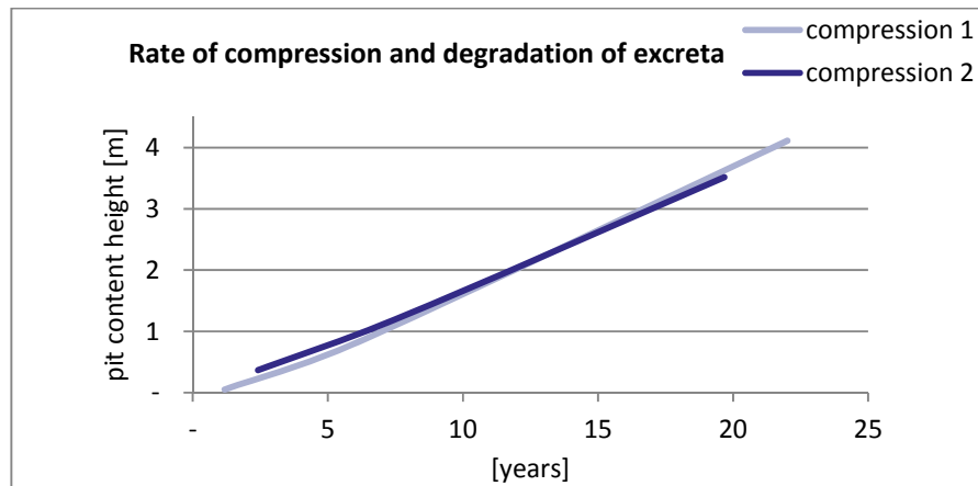
Figure 5.23: Excreta content compression over time calculated from pit input and actual height without considering rubbish input.
