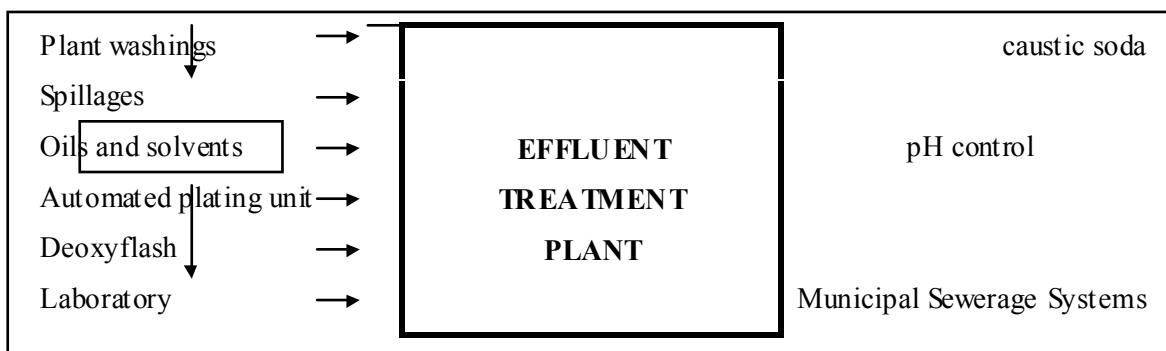
Figure C4.3: Effluent treatment plant at Company B.
