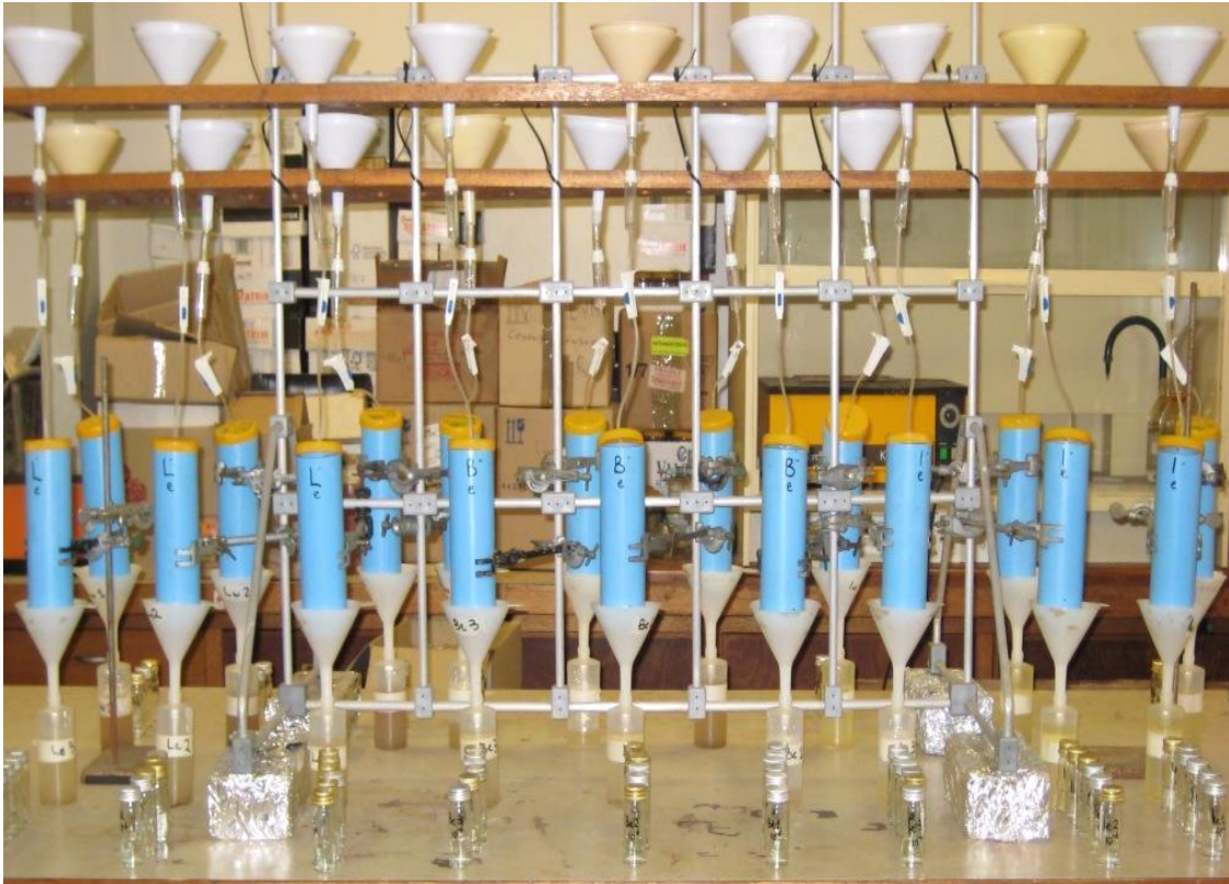
Plate 3.2 Soil leaching columns laboratory set-up.
