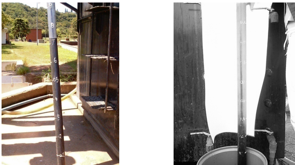
Figure 3.7: Core Sampler filled with compartment 1 sludge (left) and compartment 8 sludge and supernatant (right)
