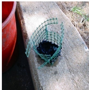
Figure 5.2: Modified outlet of the ABR showing mesh for preventing coarse solids entering the flow meter.
