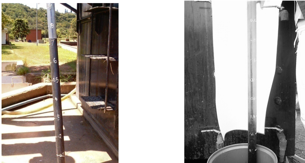
Figure A2. 1: Core Sampler filled with compartment 1 sludge (left) and compartment 8 sludge and supernatant (right)
