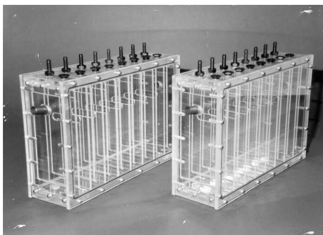
Figure 3.1: 10 ℓ Perspex laboratory-scale ABRs showing inlet, internal baffles, gas vents and sampling ports ((Bell, 2002))
