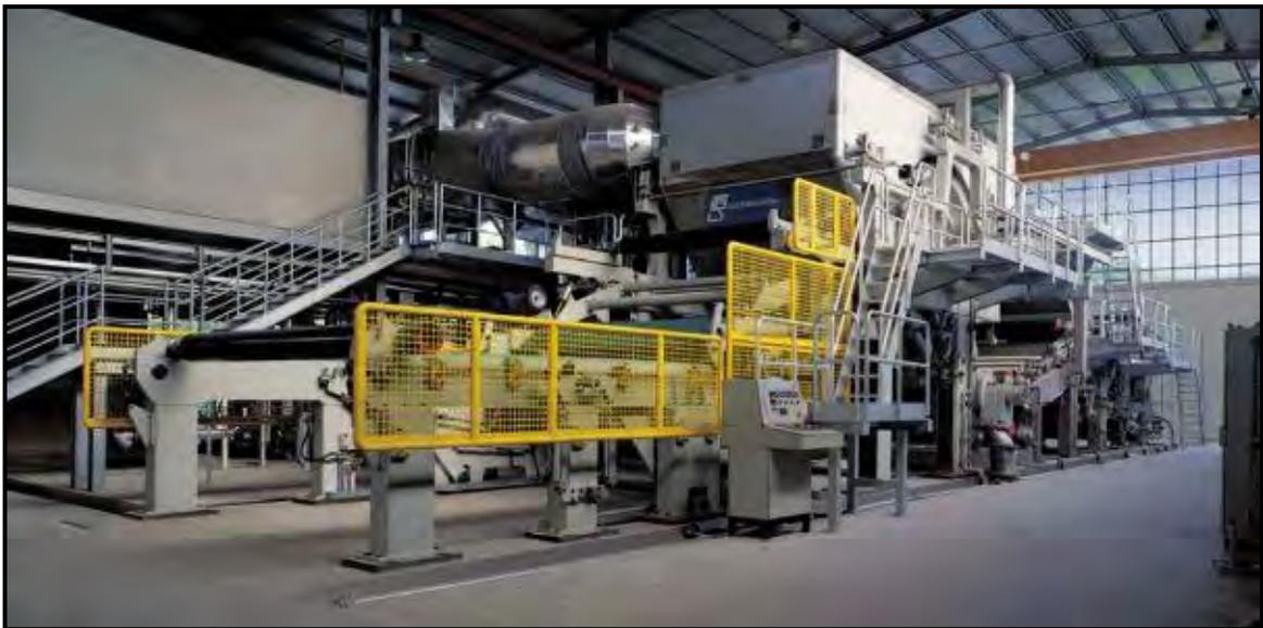
**Figure 2-2: Image of a tissue machine (headbox to the Yankee) ([www.paperonweb.com](http://www.paperonweb.com))**
