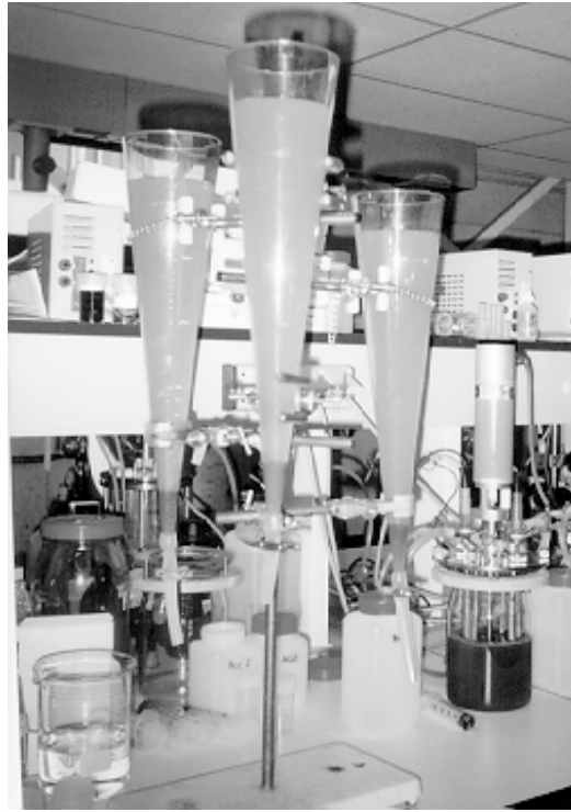
Figure 4-1 : Photo of settling test using Imhoff cone.
