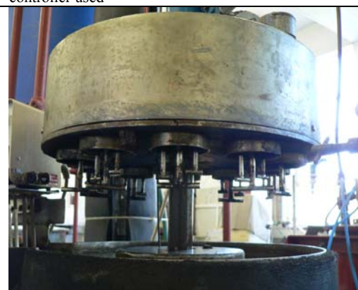
Fig 4.2 : Front view of the stirrers with a temperature controller used
