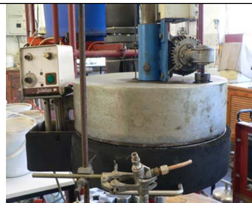
Fig 4.2 : Front view of the stirrers with a temperature controller used
