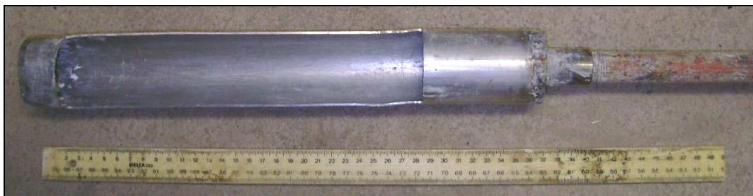
Figure A-6 Top view of corer, measured against a 50 cm ruler.
