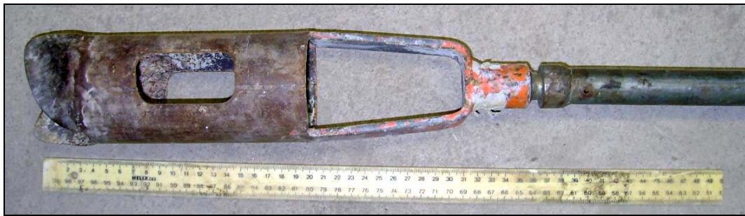
Figure A-4 Modified bucket auger, measured against a 50 cm ruler.
