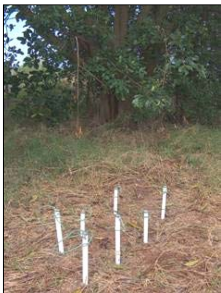
Figure A-3 Photograph of redox electrodes installed at Site 21 at Dam 2.
