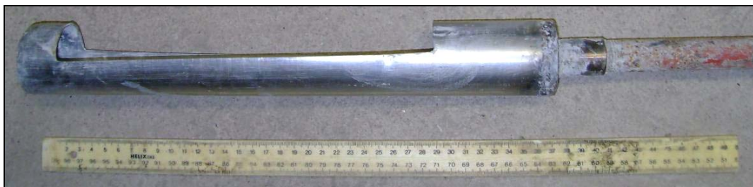
Figure A-5 Side view of corer, measured against a 50 cm ruler.
