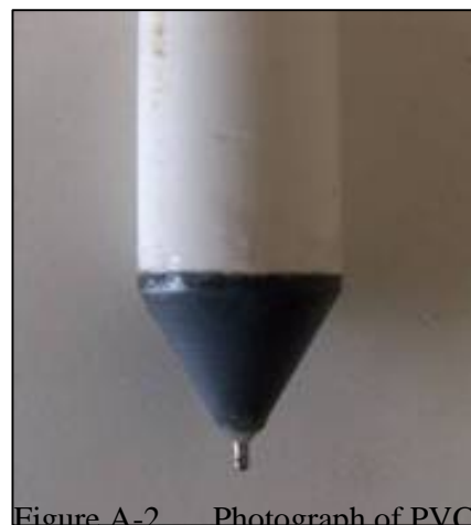
Figure A-2 Photograph of PVC cap and tubing protecting the electrode.
