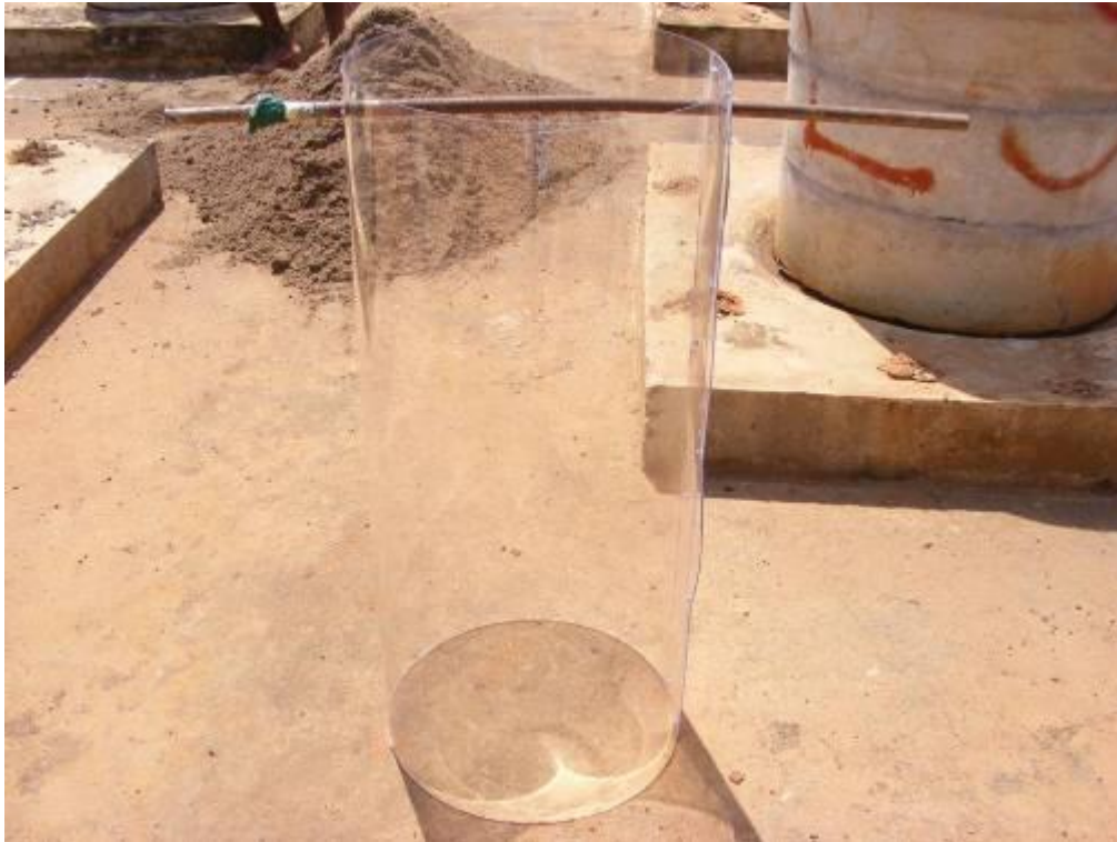
Figure 2.4: Polycarbonate cylinder used to achieve the desired application of faecal sludge.
