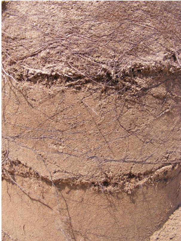
Figure 3.21: Exposed sand profile of a control column in which E. grandis was grown. Markings across the profile indicate where concrete rings were joined.
