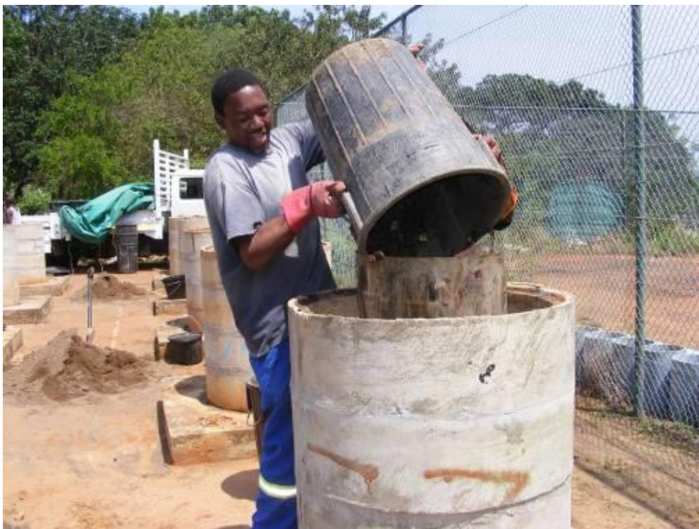
Figure 2.5: Application of faecal sludge. Sludge was applied directly into the cylinder until the desired level was reached.
