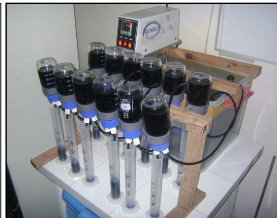
Figure 171: SMA setup in Yogyakarta with twelve displacement bottles and measuring cylinders, water-bath with temperature control containing the reactor bottles is in the background
