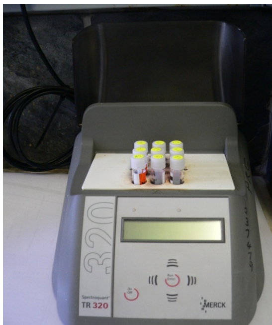
Spectroquant Heating Block (TR320-Merck)
