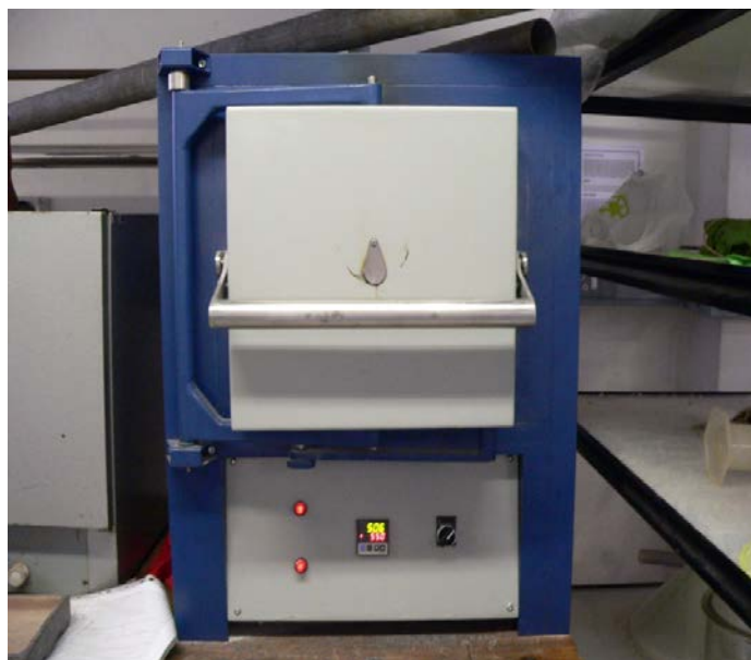
Furnace (E160) - Temperature: 550 °C
