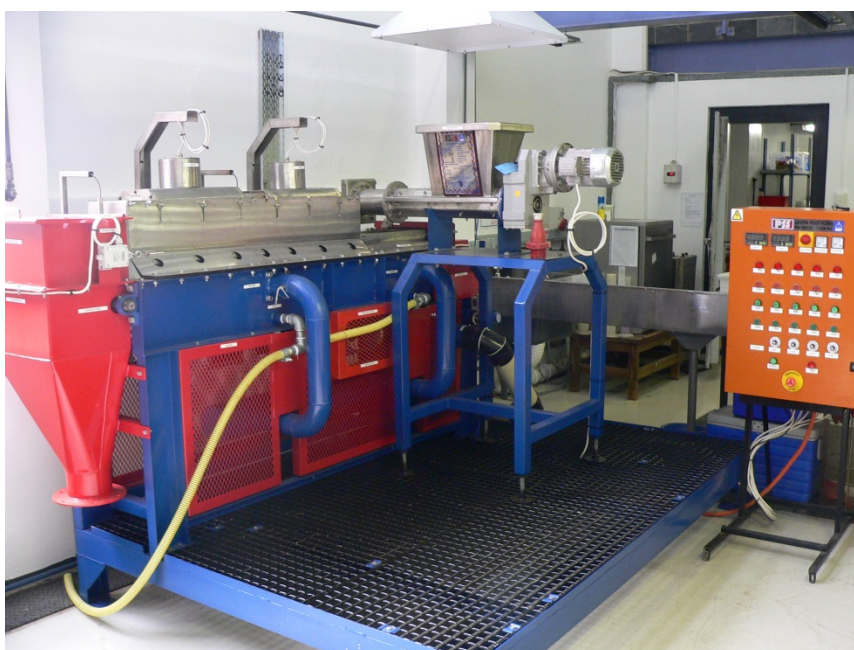
LaDePa (Latrine dehydration and pasteurisation) machine (laboratory scale)
