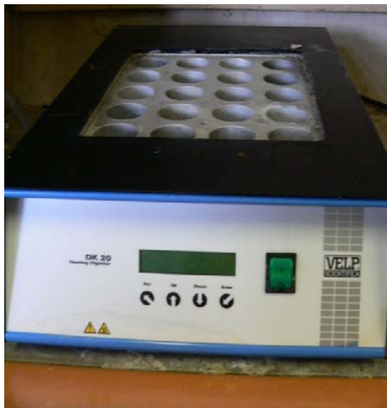
Heating Block Digester (DK20-VELP)
