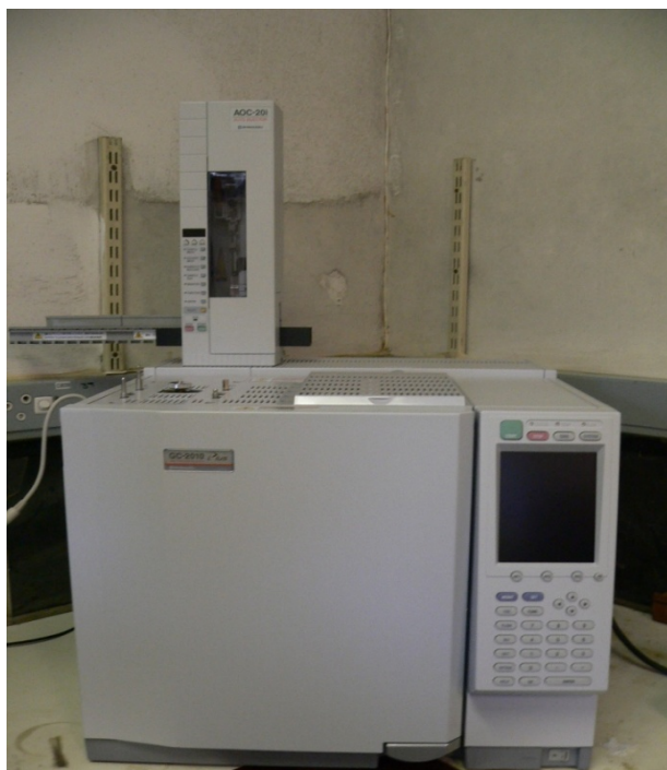
Gas Chromatograph (GC-2010 Plus-Shimadzu)
