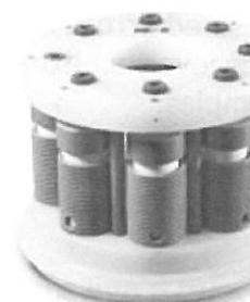
Reference vessel must be placed in position number one on rotor plate.
