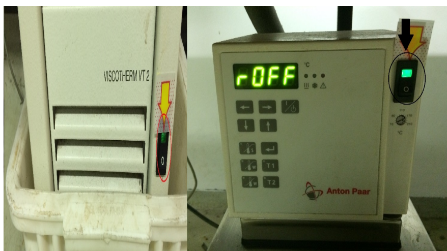
Figure 2: Switch on the tower under the table
