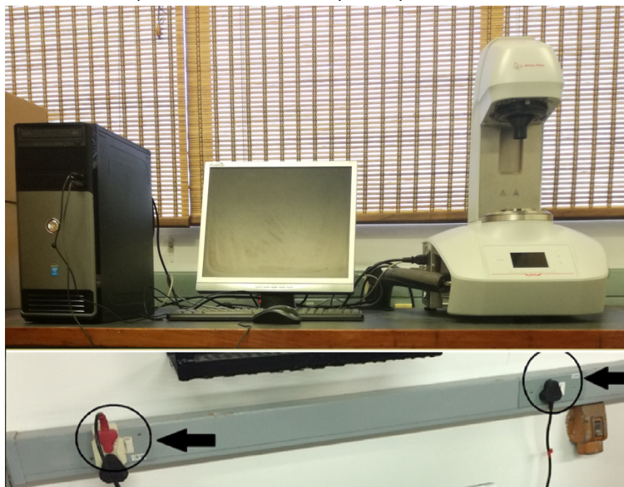
Figure 1: Check that the instrument is in good condition then switch on the plugs on the wall
