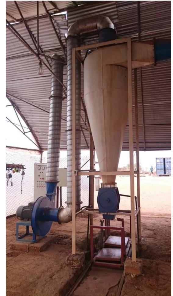
Cyclone to recover the dried material
