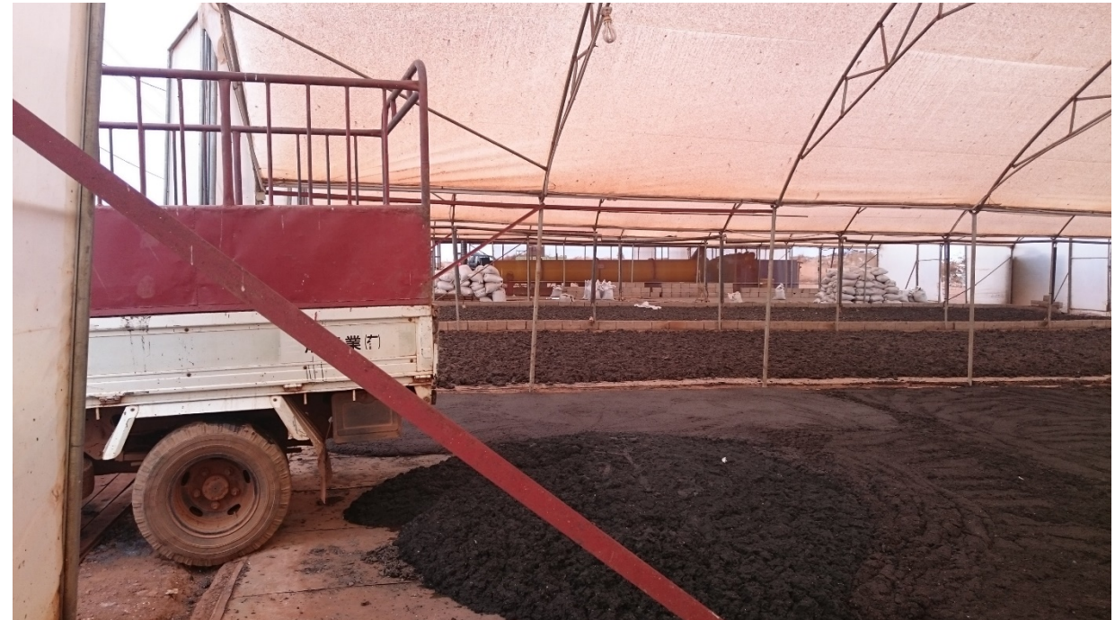
Discharge of dewatered faecal sludge inside the greenhouse
