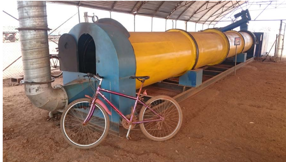
Rotary drum drier (convective drying from the gases of combustion)
