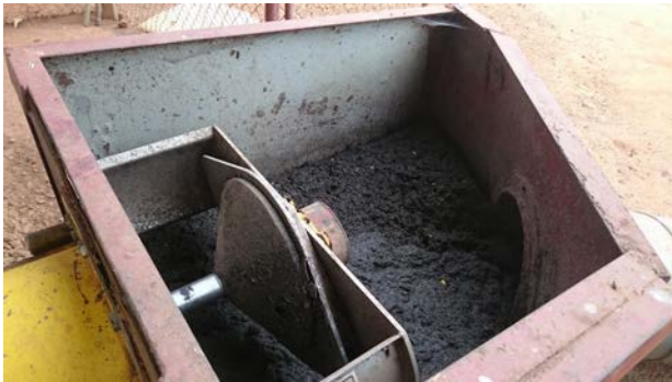
Outlet of the mechanical dewatering machine
