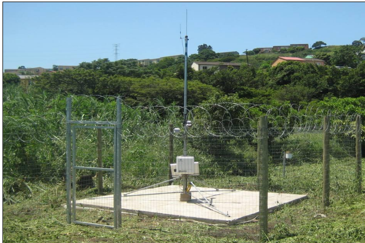
Figure 3: Automated weather station to monitor weather conditions at Newlands Mashu.
