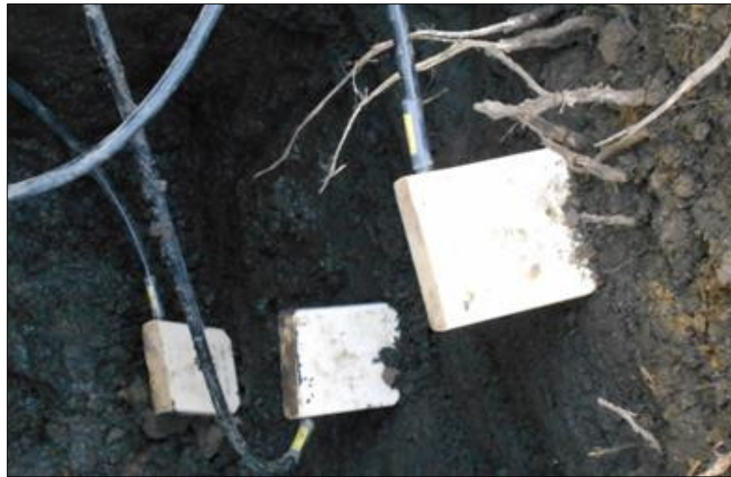
Figure 4: Campbell scientific soil reflectometers used to monitor soil moisture content.
