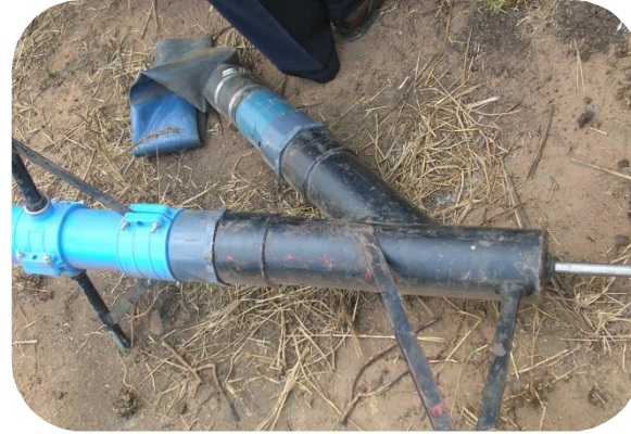
Human powered: improved manual – e.g. Gulper, eVac
