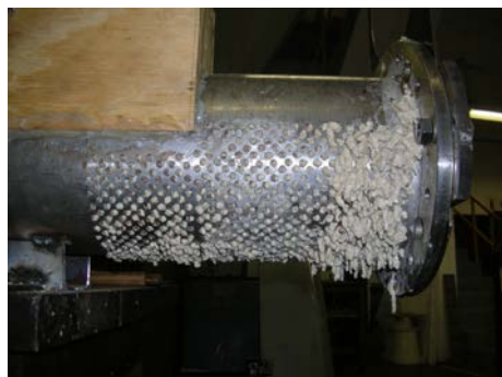
Prototype system for separating faeces and rubbish and extruding faeces for drying
