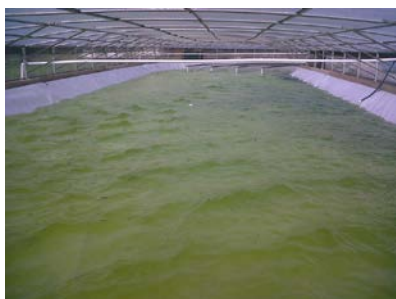
Algae being cultivated in the 300 000 L raceway pond at Kingsburgh wastewater treatment works
