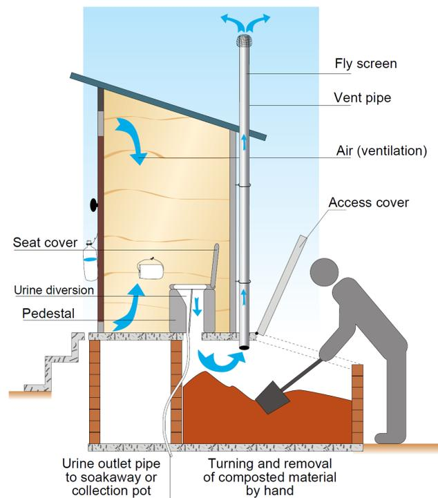
Figure 1: Schematic of a Urine Diversion Toilet (2)
