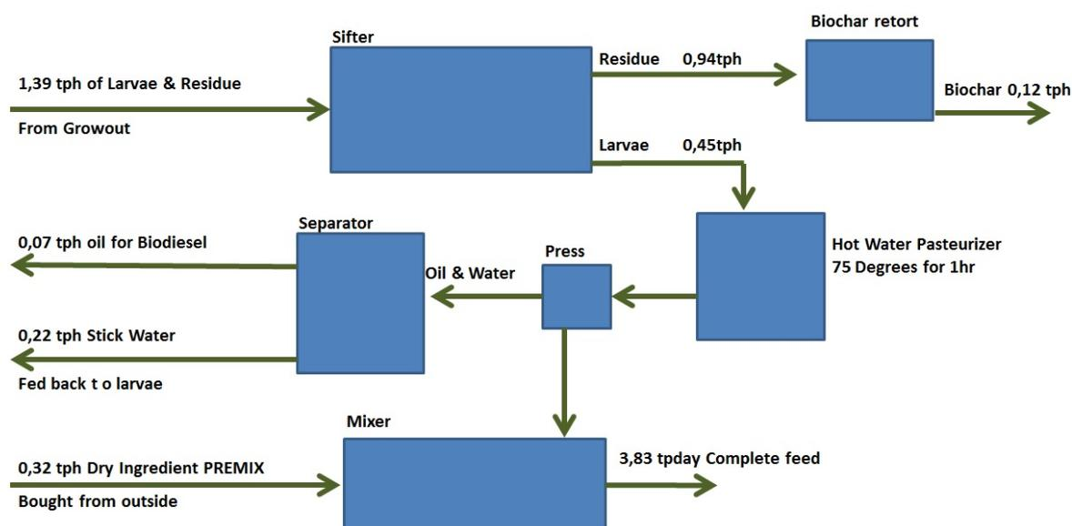
Figure 4: BSF Processing Flowchart
