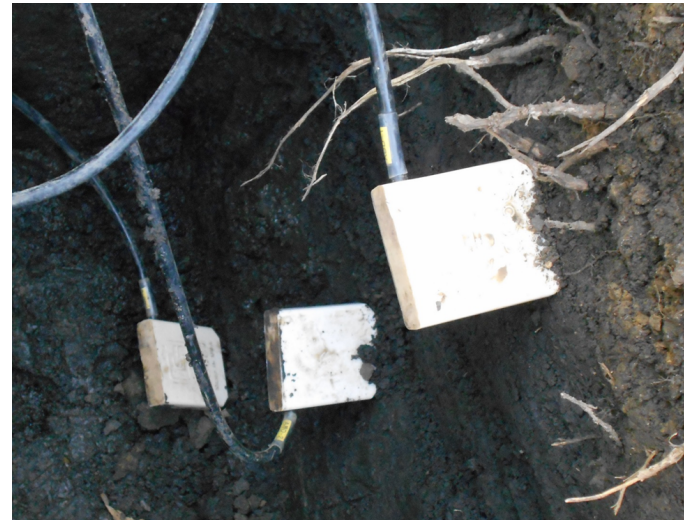
CS 650 soil water content reflectometers
