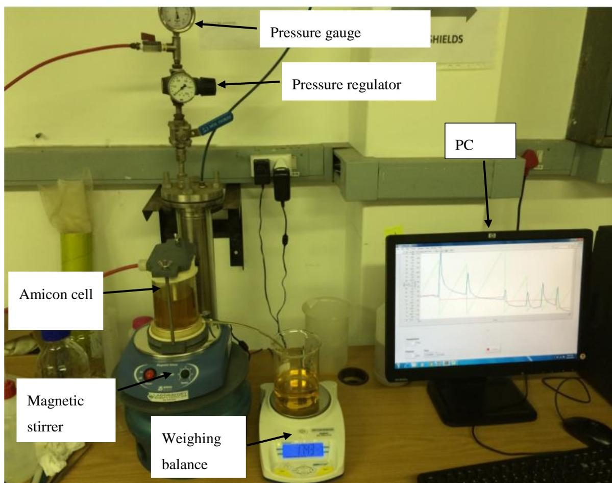
Figure 3-2: Experimental setup
