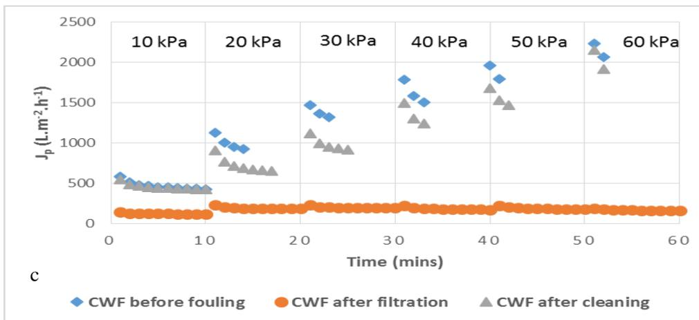
**Figure B 2: Figure B 1: Flux vs time at different TMP during clean water fluxes (filtration of deionised water) for: a) case 1, b) case 2 and c) case 3**
