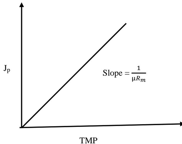
**Figure 2-3: Plot of flux versus transmembrane pressure for the determination of permeability**
