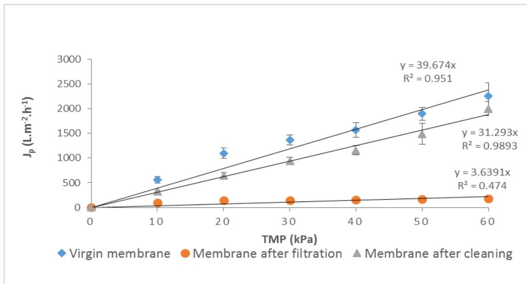
**Figure 4-2 Permeate flux as a function of the transmembrane pressure for the virgin membrane, membrane after filtration and after cleaning during the clean water flux tests for case 1**
