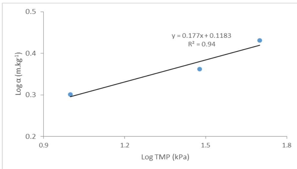
**Figure 4-8: Plot of  $\log \alpha$  vs.  $\log$  TMP to get the compressibility index of the cake formed during diluted urine filtration**
