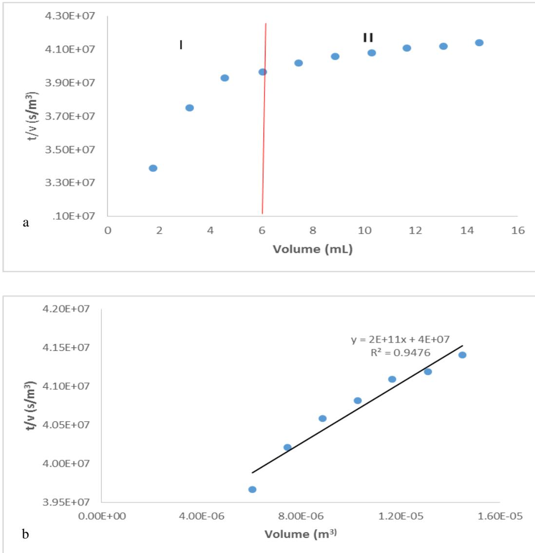
**Figure E 1: Plots of time/volume versus volume at 50 kPa of stored urine 60-10 kPa for a) curve and b) Linear regression**
