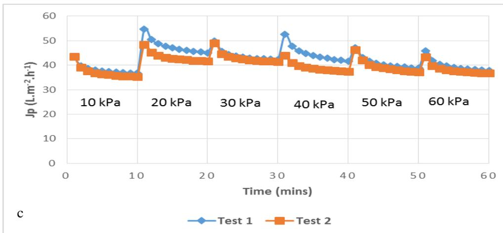
**Figure B 1: Flux vs time during at different TMP steps during stored urine filtration for: a) case 1, b) case 2 and c) case 3**
