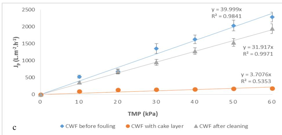
**Figure D 1: Clean water flux tests for the membranes used in Case 1 – a) Membrane 1 ; b) Membrane 2 ; c) Membrane 3**
