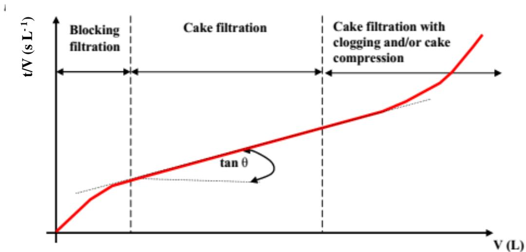
Figure 2-4: Filtration time divided by the filtrate volume ( $t/V$ ) as a function of the filtrate volume ( $V$ ) (Boerlage et al., 2003)
