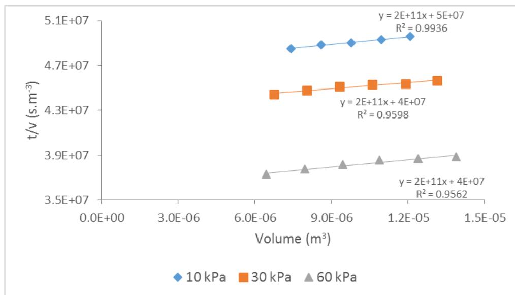
Figure 4-6: Summary of plots of  $t/v$  vs.  $V$  at different pressures for case 1
