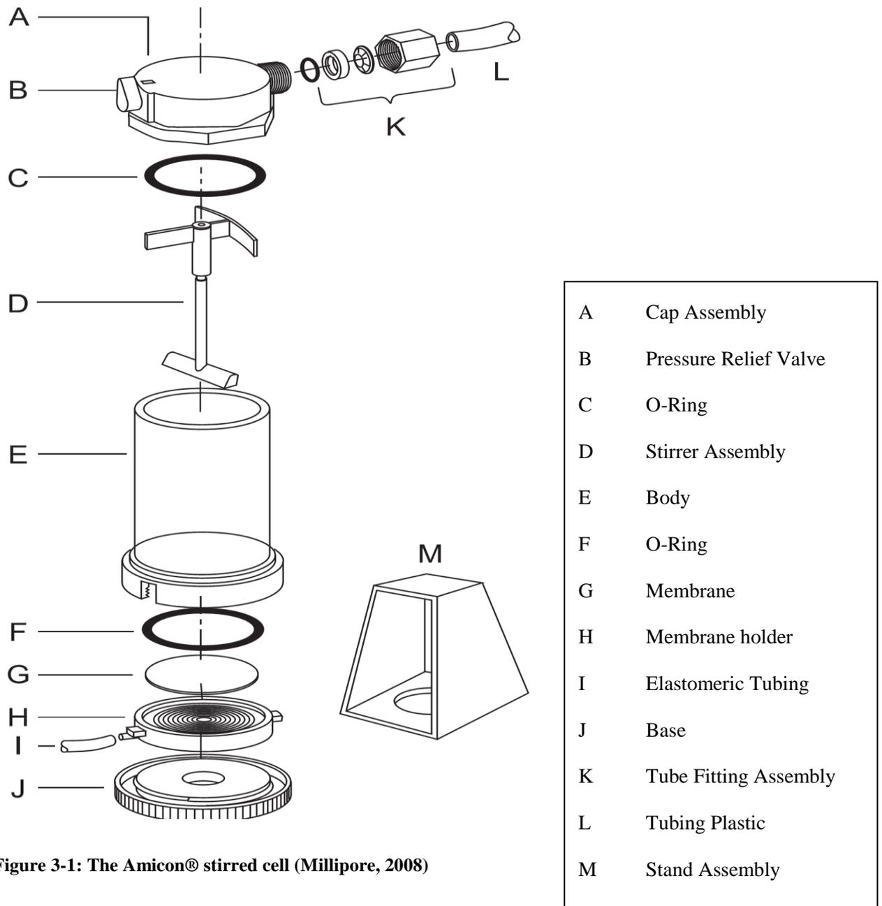
**Figure 3-1: The Amicon® stirred cell (Millipore, 2008)**
