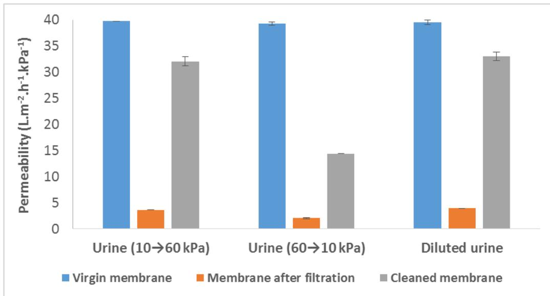
Figure 4-3: Permeability of the membrane before filtration, after filtration, and after cleaning
