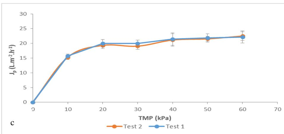
**Figure C 1: Permeate flux at 20°C obtained during urine filtration for case 1 - a) membrane 1 ; b) membrane 2; c) membrane 3**
