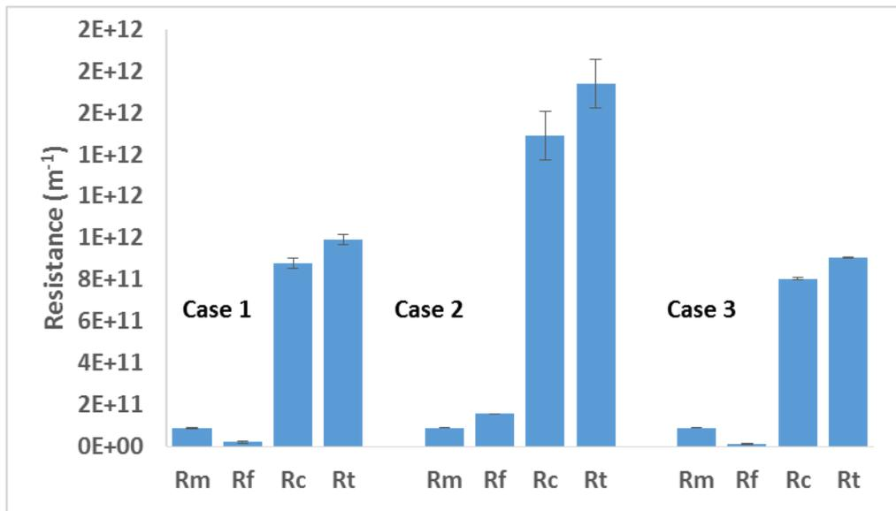
**Figure 4-4: Membrane hydraulic resistances during filtration for the 3 experimental cases**
