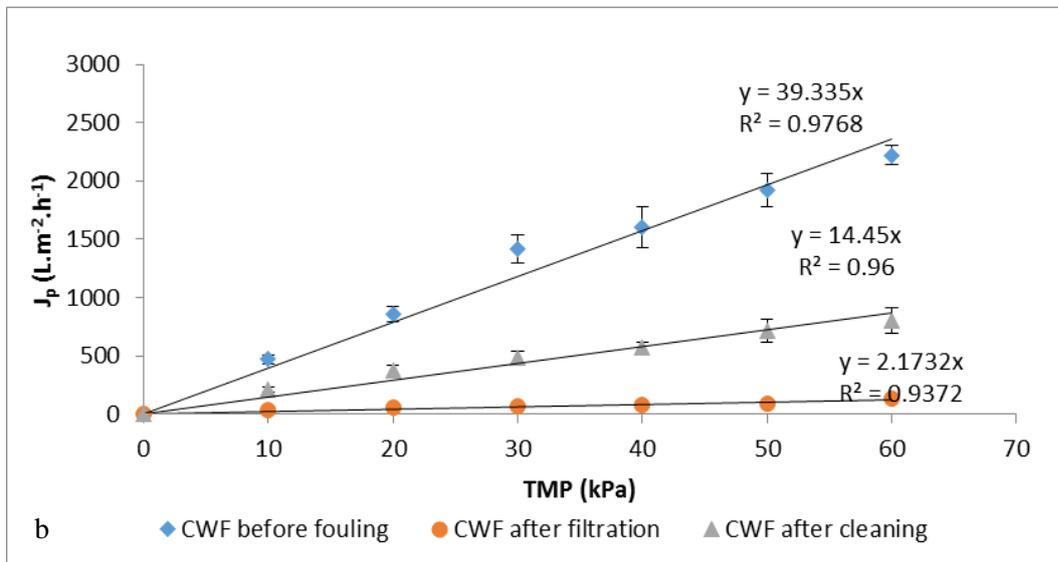
Figure D 2: Clean water flux tests for the membranes used in case 2 – a) Membrane 4 ; b) Membrane 5
