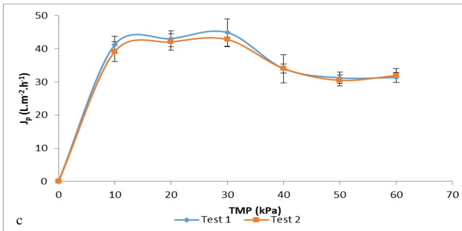
Figure C 3: Permeate flux at 20°C obtained during urine filtration for case 3 - a) membrane 6 ; b) membrane 7; c) membrane 8
