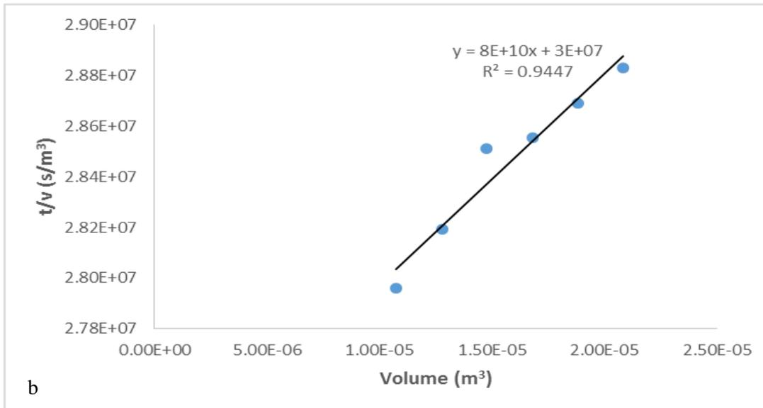
**Figure E 2: Plots of time/volume versus volume at 50 kPa of stored diluted urine 10-60 kPa for a) curve and b) Linear regression.**
