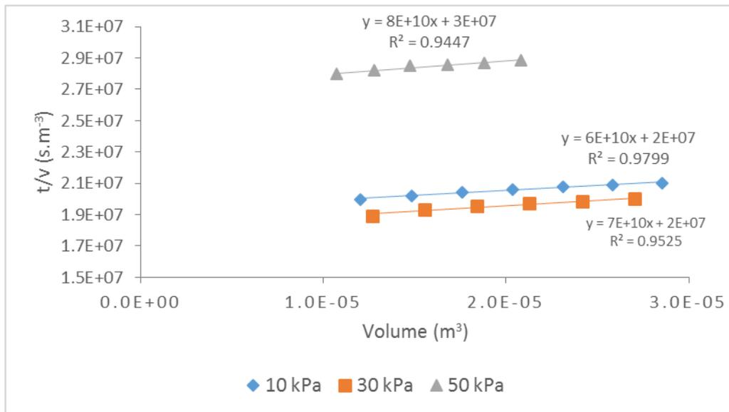
**Figure 4-7: Summary of plots of  $t/v$  vs.  $V$  at different pressures for case 3**
