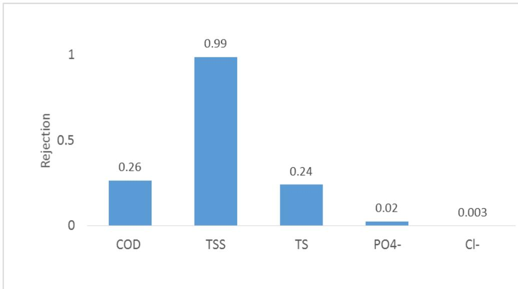
Figure 4-10: Rejections during urine filtration
