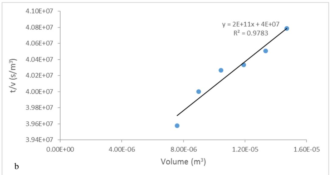
**Figure 4-5: Plots of  $t/V$  versus volume at 50 kPa of stored urine 10-60 kPa for a) the entire curve and b) Linear regression.**
