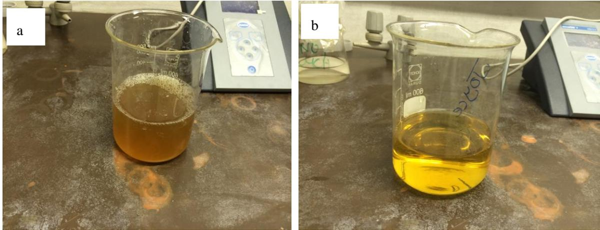
**Figure 4-11: Photograph of stored urine - (a) before filtration (feedstock) (b) after filtration (permeate)**
