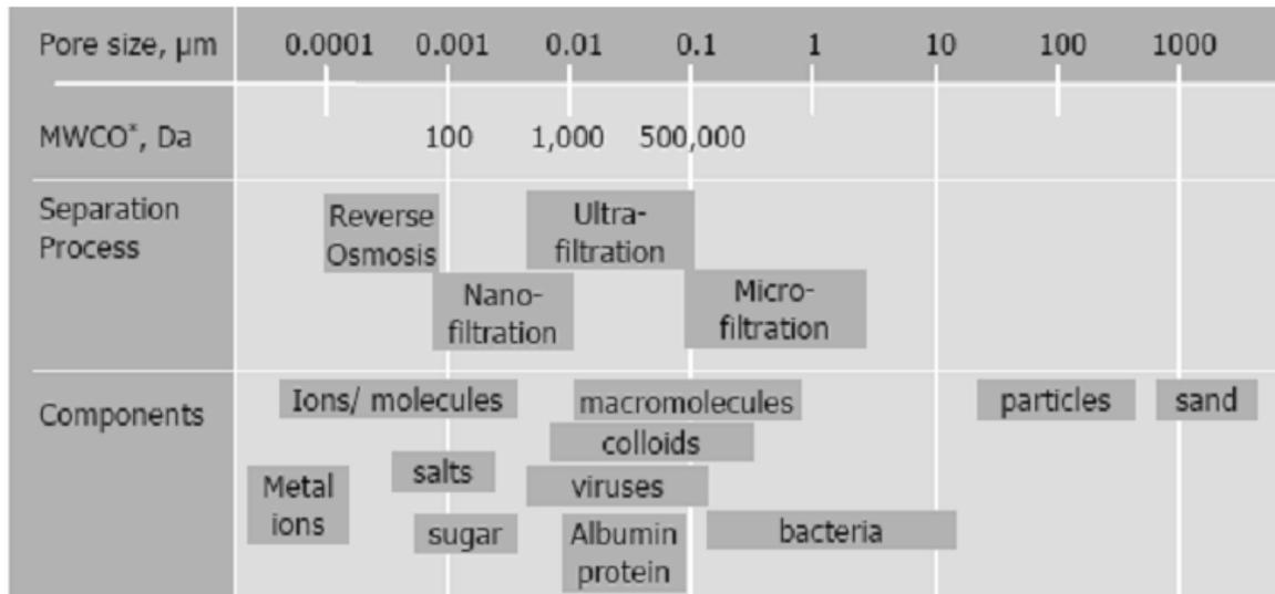
**Figure 2-1: Classification of pressure driven membrane processes in terms of Molecular Weight Cut-off (Pillay, 2011)**
